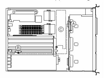
Figure 31: Connecting to a Full Height PCI SCSI Controller
